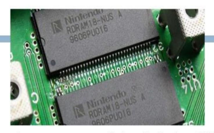
random access memory: Designed by Rambus, RDRAM uses a Rambus in-line memory module (RIMM), which is similar in size and pin configuration to a standard DIMM. RDRAM memory chips work in parallel to achieve a data rate of 800 MHz, or 1,600 Mbps. Since they operate at such high speeds, they generate much more heat than other types of chips.
